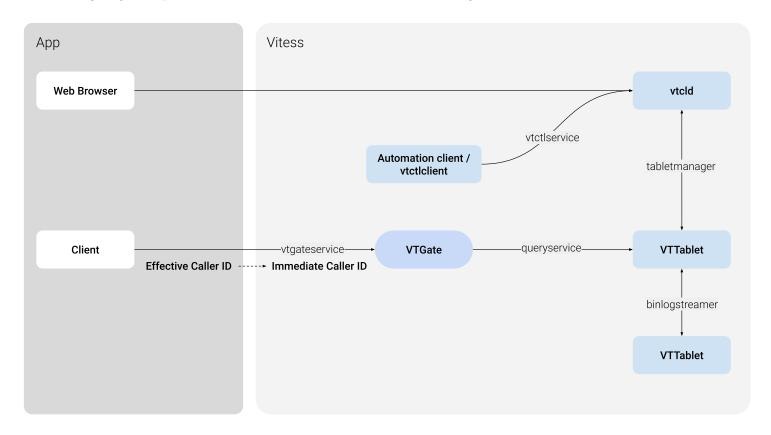
Figure 3: Vitess Transport Security Model Diagram
