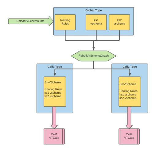
Figure 4: VSchema Architecture
